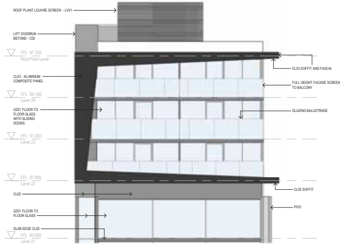
① North Elevation - Crown Detail 1:100
